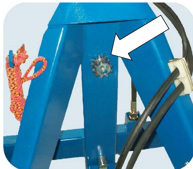
Fig. 11d Position of the Additional Spur Gear for Wrapping with 20" Film.
