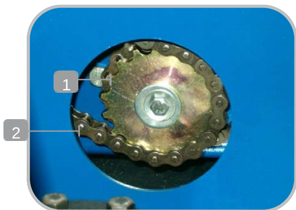
Fig. 11c Spur Gear Replacement. 1-Spur Gear Z-19; 2-5/8" Chain
